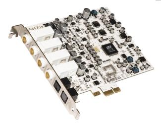
The MAYA44 XTe is a high quality 24-bit / 96 kHz 4-in / 4-out PCIe audio interface, providing a number of powerful and amazing features optimized for home recording on a professional quality level and for various DJ applications.
