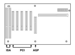
typical PC motherboard slot configuration
