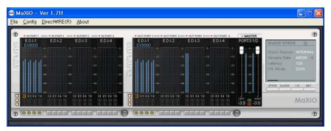
In many typical setups you would use output 1/2 of the first port (e.g. the first EX8000) as master output. Via the monitoring buttons (see below) you can then mix all signals to this stereo output.
