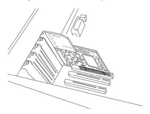
MaXiO PCI host card installed in a PCI slot
