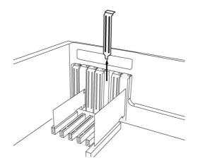
removing the PCI slot faceplate
